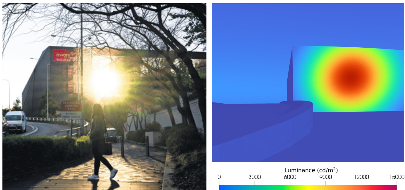
Figure 1: Winter solstice morning solar reflection off facade glazing - photograph courtesy Sydney Morning Herald (Left), Simulated luminance arriving at the viewing position (Right).
